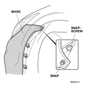
8. Attach six plastic hooks to the fenderwell and the holes of the inner fender. Repeat on the right side.
